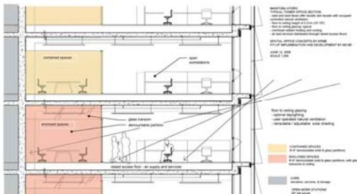
Fig 12 Typical loft sections showing daylight penetration
